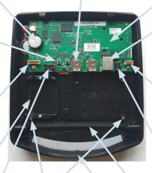
Mounting points for Reader Module Front cover fixing screw
